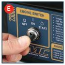
4. Turn the key start ignition (10) clockwise to the 'START' position (Fig. E).
